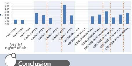
These preliminary results indicate that Coriolis<sup>®</sup>µ is a suitable method for the sampling of airborne allergen of latex by reducing the time of sampling (20 min vs. 24h) and increasing the efficiency. Furthermore, the Coriolis<sup>®</sup>µ air sampler collects any airborne particles and can also give information on specific airborne microorganisms, pollens, viruses...
